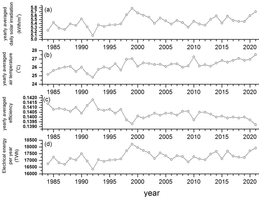
**Figure 7.** Yearly variation of several quantities. (a) Yearly averaged daily solar irradiation on a horizontal surface; (b) yearly averaged air temperature; (c) yearly averaged PV plant efficiency; (d) electrical energy provided yearly by the PV plant.
