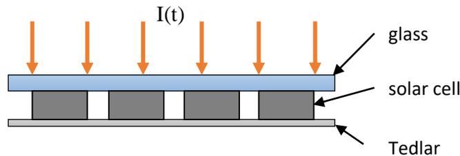
Figure 6. Cross section through opaque PV module.
