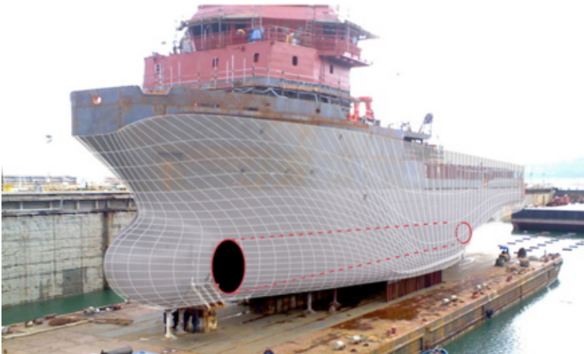
Figure 8 — Notional placing of Marine Arkiduct in conventional vessel. Base image from reference [9].
