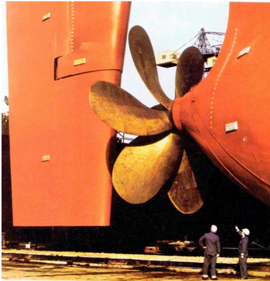
Figure 5 — Nine-metre diameter ship propeller from Hapag-Lloyd container ship [5].
