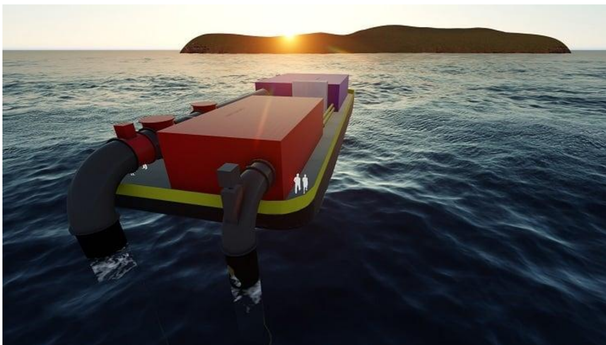
Fig 8. An OTEC system housed on a floating vessel (credits to https://maritime-executive.com/ ).
