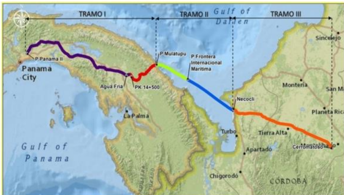
Figure 2. Panama and Columbia electrical grids linked across Gulf of Darién by underwater power-cable.
